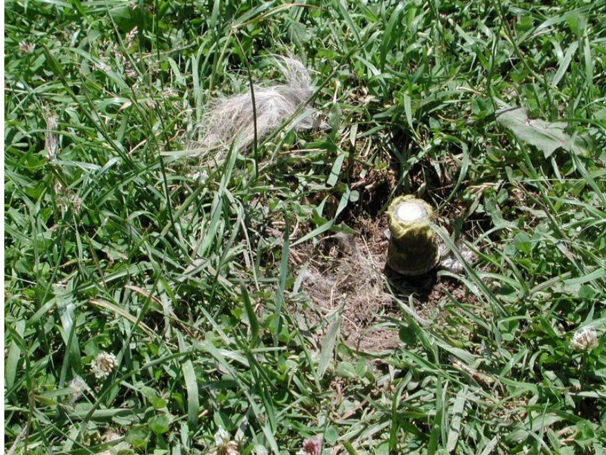
M-44 cyanide capsule, chewed. Photo Credit: U.S. Dept. of Agriculture, Wildlife Services
